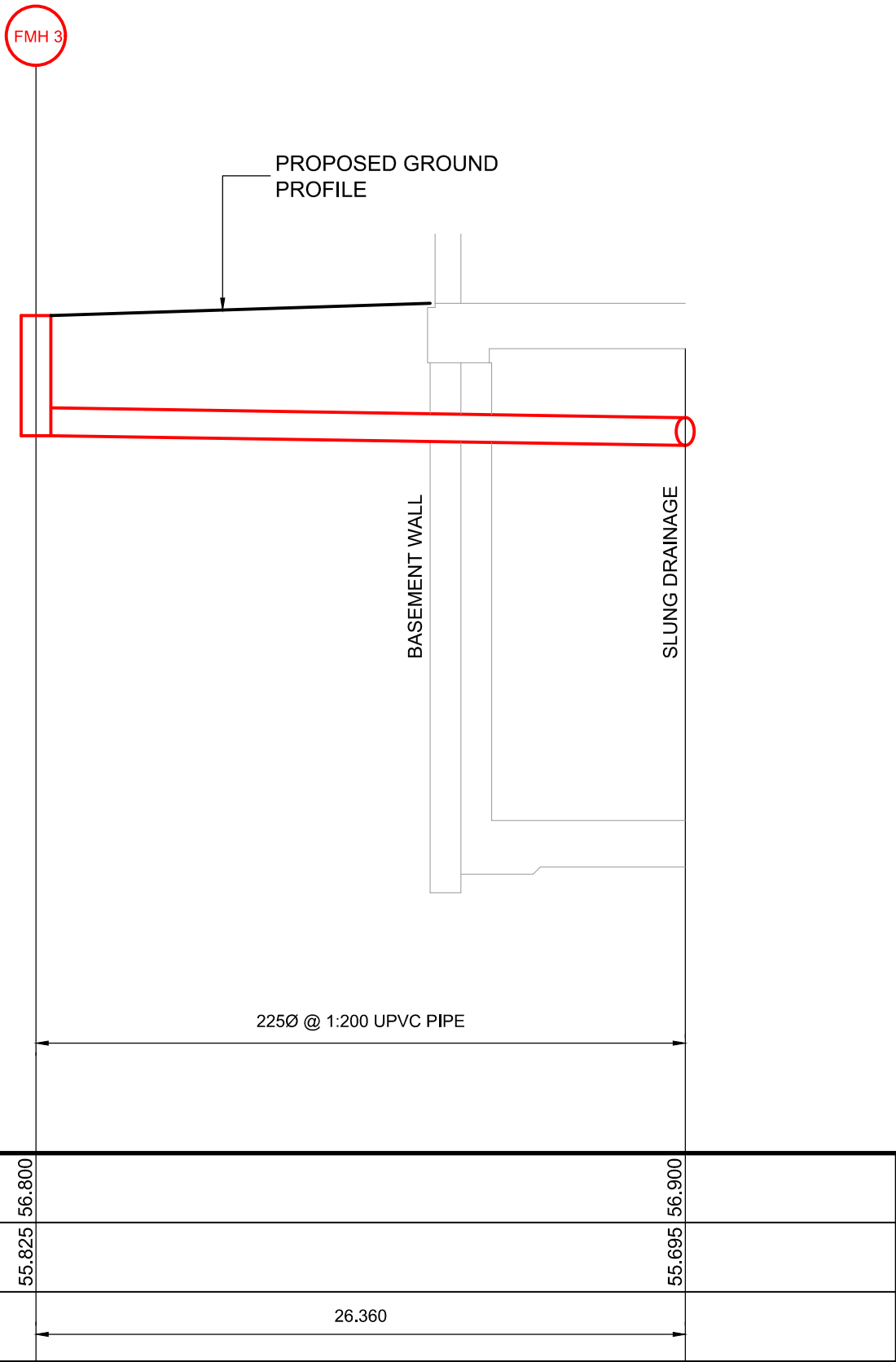
FOUL LONGITUDINAL SECTION FMH 3 TO SLUNG DRAINAGE
